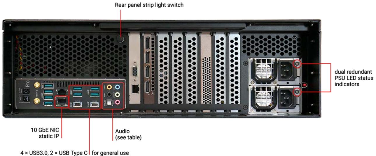
Both should be connected, since they operate in parallel. If one unit fails, the indicator light to the right of the failed socket will go to yellow and emit a high-pitched beeping sound. If only one PSU is connected, the other's indicator will show amber. Green LEDs indicate healthy PSUs.
