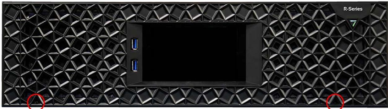
After removing the two screws, pull the fascia forwards and straight off the unit. It is retained by four push-fit fasteners. If the fascia sides are inaccessible, plastic hooks are provided to pull the fascia off (see [Installation](#) <sup>5</sup> ).
