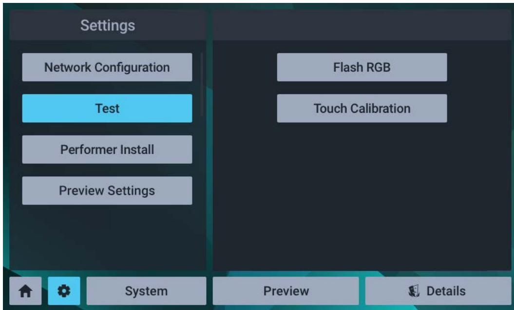
The **Test** button has two functions, to cycle all outputs once through solid red/green/blue, and to calibrate the touch function.
